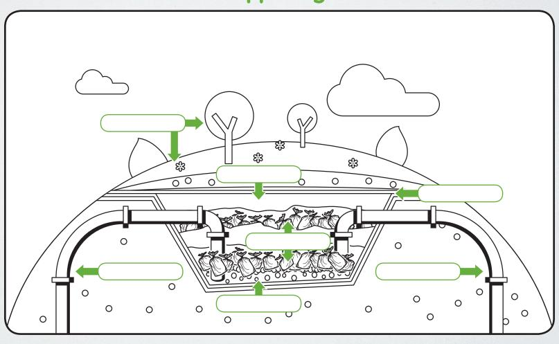
Leachate Pipe • Plastic Liner • Gravel • Soil • Grass and Trees • Gas Pipe • Waste
